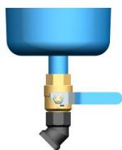
首先安装法兰接头 Install flange joint
